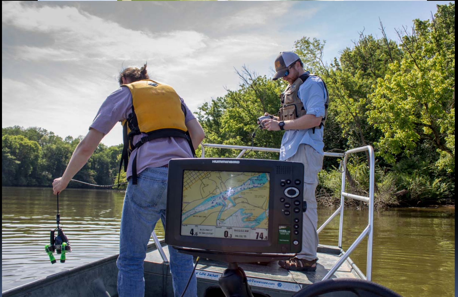
Side-scan sonar survey with Humminbird © fish-finder unit
